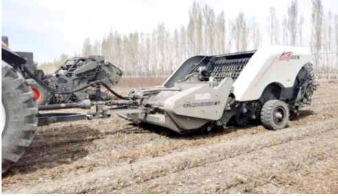
图 21 4JMLQ-210 型秸秆还田残膜回收联合作业机 Fig. 21 4JMLQ-210 type cotton straw smashing and plastic film recycling combined operation machine
